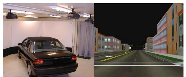
FIGURE 3 Driver simulator vehicle and configuration (left) and sample simulated visual world (right).
