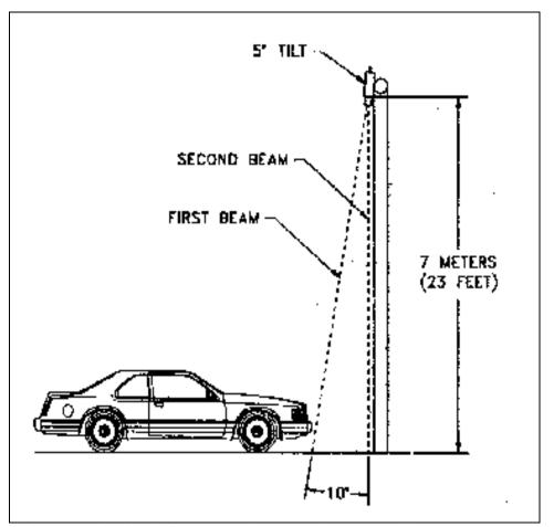
FIGURE 2 Active-infrared device mounting angle (6).
