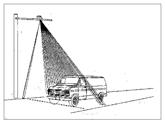
FIGURE 1 Typical active-infrared scan pattern (6).
