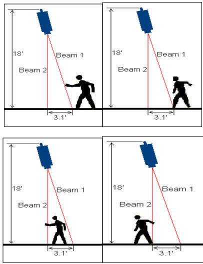
FIGURE 7 Pedestrian movement underneath the sensor.
