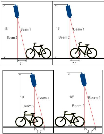
FIGURE 6 Bicycle movement underneath the sensor.
