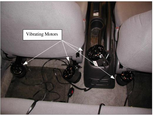
FIGURE 4 Location of Vibrator Motors Inside Vehicle Cab.
