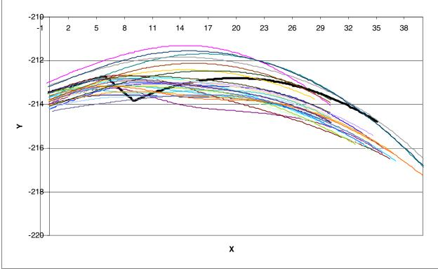
Vehicle Paths, Centerline Rumble Strip, Database 2, Module 1, Scenario 6. FIGURE 5 Sample 'x'-'y' Vehicle Paths Plots at Centerline Rumble Strips.
