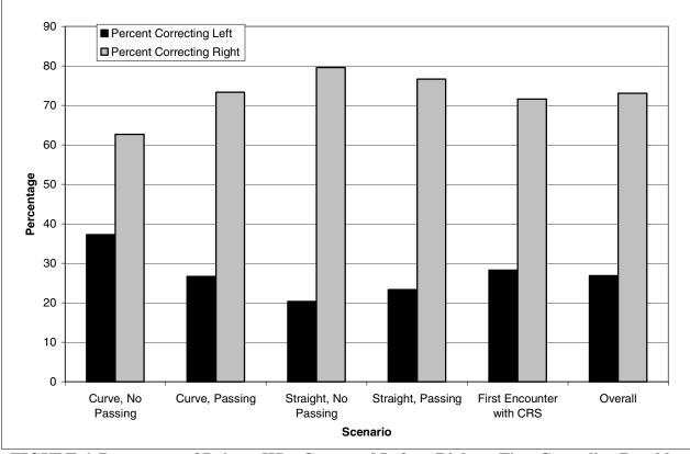
FIGURE 6 Percentage of Drivers Who Corrected Left or Right at First Centerline Rumble Strip Encounter.
