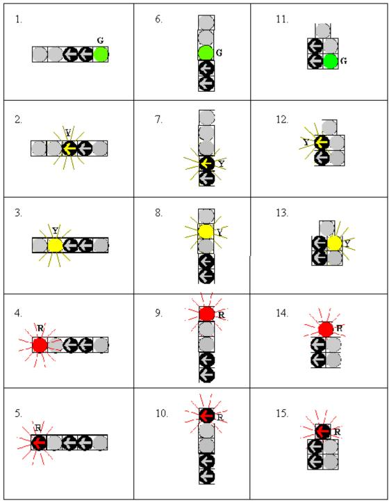
Permissive Indications: R = FLASHING RED Y = FLASHING YELLOW G = STEADY GREEN
