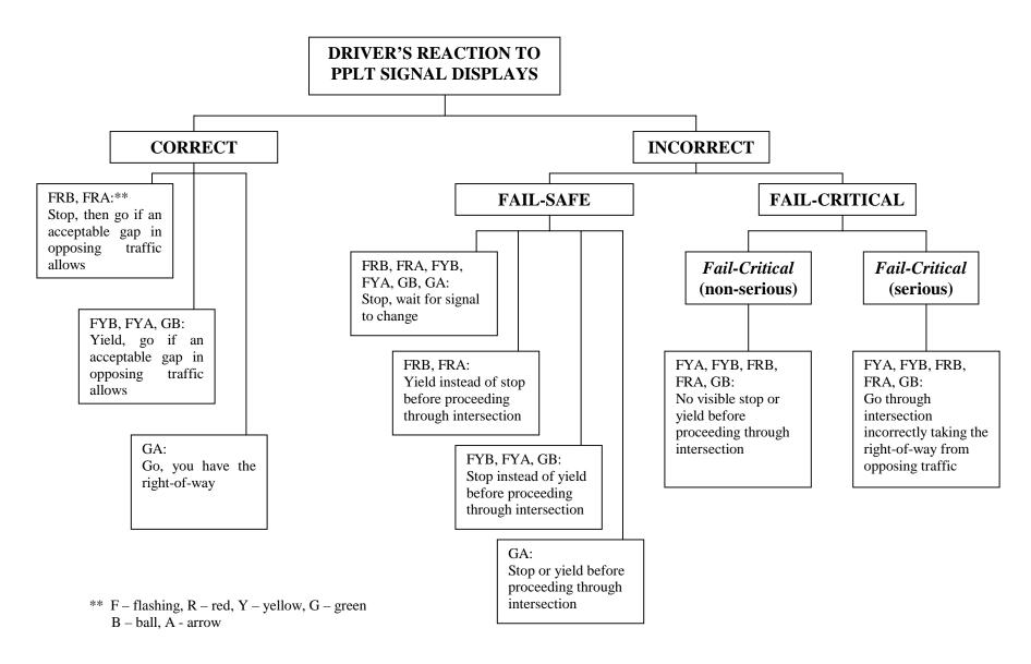
Figure 3 Response Categories for Driver Actions in Simulator Experiment
