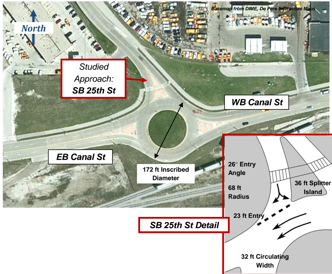
Figure 4.2. Canal St Site Configuration
